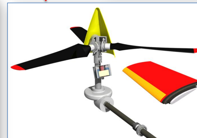
Propellers Controlable pitch Composite structure
