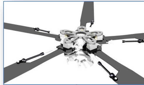
Rotor Hub Hingeless design
